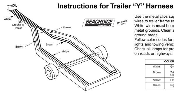
Use the metal clips supplied in this kit to clip the wires to trailer frame rails.
